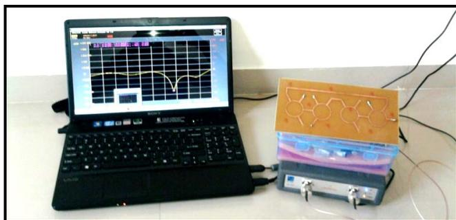
Fig. 2. The MCNS testing using the ELAD SNA-2550
