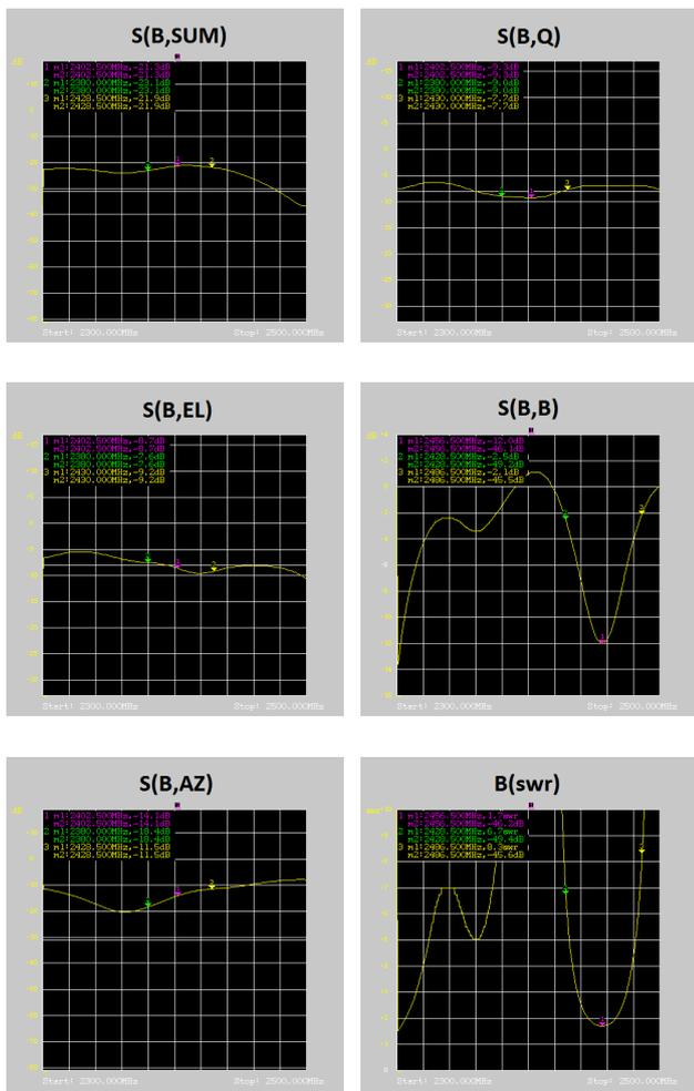
Fig. 4. SWR, Return loss and output results for Input B with different outputs
