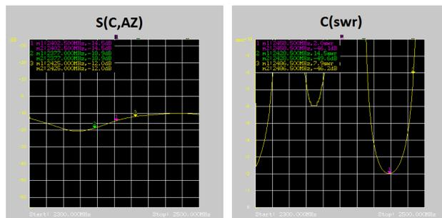
Fig. 5. SWR, Return loss and output results for Input C with different outputs
