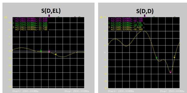
Fig. 6. SWR, Return loss and output results for Input D with different outputs
