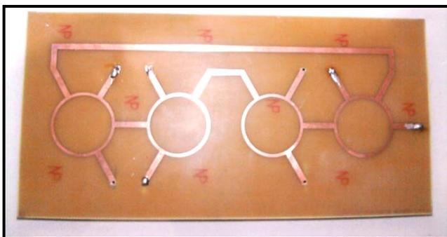
Fig. 1. Mono-pulse Comparator Network Systems (MCNS) with hybrid rings.
