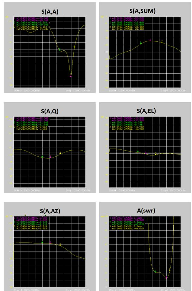
Fig. 3. SWR, Return loss and output results for Input A with different outputs
